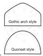
of structure is that the walls go straight up, allowing equipment such as rototillers or cultivators to work closer to the wall. The traditional Quonset style usually begins its curving arch right at soil level.
